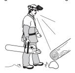
Take the utmost care when cutting through branches or logs that are in tension. A log or branch that is in tension can suddenly spring back into its natural position before or after you cut it. If you stand on the wrong side or start cutting in the wrong place it may strike you or your chain saw, so that you lose control. Both situations could cause serious injury.
